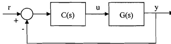
If the controller  $C(s)$  is of proportional type (i.e.  $C(s)=K$ , a constant), find the range of  $K$  so that the closed-loop system is stable. (7%)
