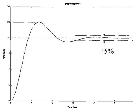
$$\text{Settling time } (\pm 5\%): t_s = \frac{3}{\zeta\omega_n}$$
