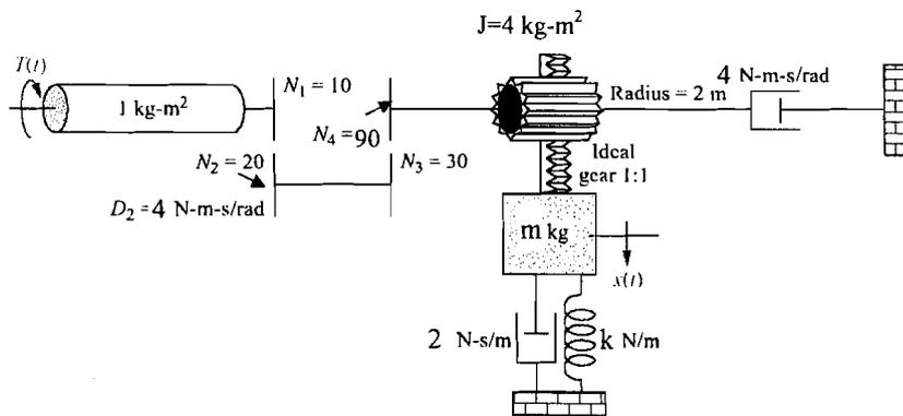
6. Find the transfer function  $T(s)=Y(s)/R(s)$ , determine the system type and find the steady state error with respect to an input  $R(s)=10/s$ . Is this system a minimum phase one? Stable? (15%)
